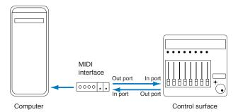
*Important*: It is recommended that you do not daisy-chain other MIDI devices via MIDI through to the MIDI In or Out ports used by control surfaces. Daisy-chaining can result in errors and other problems due to the amount of data transmitted in real time.
