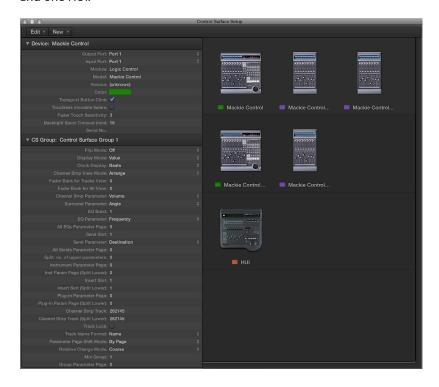
The top row, consisting of the Mackie Control #1, Mackie Control XT #1, and Mackie Control XT #2, forms a single control surface group with 24 channels. Mackie Control #1 controls channels 1 to 8, XT #1 controls channels 9 to 16, and XT #2 handles channels 17 to 24.
