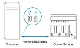
*Important:* It is recommended that you connect FireWire and USB devices directly to your computer, rather than through a hub. Daisy-chaining devices can result in errors and other problems, due to the amount of data transmitted in real time.
