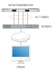
The switch should have a bandwidth for handling incoming traffic equal to or greater than that of the link aggregate (logical link) you define on your server.
