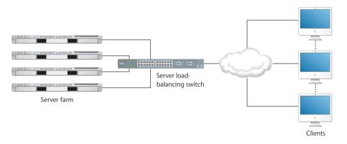
**Note:** A load-balancing device must be able to handle the aggregate (combined) traffic of the servers connected to it. Otherwise, the device becomes a bottleneck, which reduces the availability of your servers.
