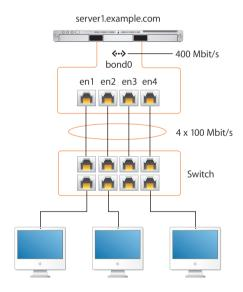
Link aggregation also allows you to take advantage of existing or inexpensive hardware to increase the bandwidth of your server. For example, you can form a link aggregate from a combination of multiple 100-Mbit/s links or 1-Gbit/s links.
