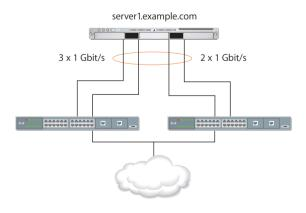
For example, you can connect two links of the link aggregate to the master switch and the remaining links to the backup switch. As long as the master switch is active, the backup switch remains inactive. If the master switch fails, the backup switch takes over transparently to the user.
