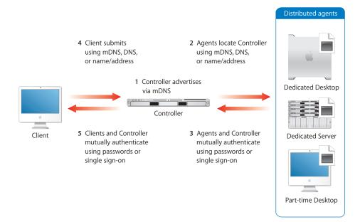
The primary components of a computational grid perform the following functions:
