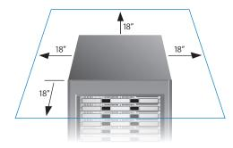
You should have enough space to open the rack's door, slide out systems, and perform other routine maintenance tasks.
