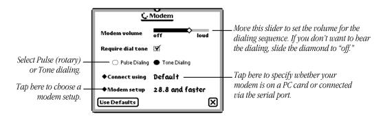
In the modem setup list, choose a modem that's similar to yours. The modem choices depend on the model of Newton device you're using. Consult your modem's manual for further information. (See the Appendix to learn how to obtain information on Newton-compatible modems.)
