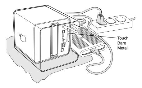
**Important:** To avoid electrostatic discharge, always ground yourself by touching the bare metal before you touch any parts or install any components inside the computer. To avoid static electricity building back up in your body, do not walk around the room until you have completed the installation and closed the computer.
