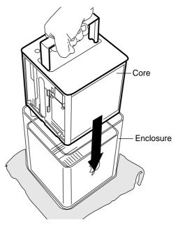
2 With a flat hand, press down on the latch until it locks into place. Firmly press the core to ensure it is fully secured within the enclosure.
