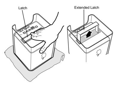
7 Gently pull the core from the computer enclosure and place the core on a soft cloth.
