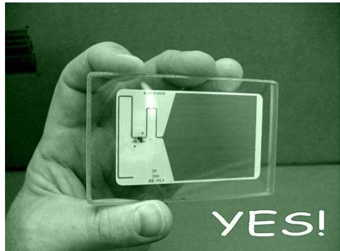
Body-blocking of the GMWS Glass-Mounted Windshield Tag, for use with AWID's LR-911 Long-Range Reader, can be eliminated by holding the glass rectangle as shown in the photograph above. This method of holding the tag keeps the hand behind the glass, away from the reader.
