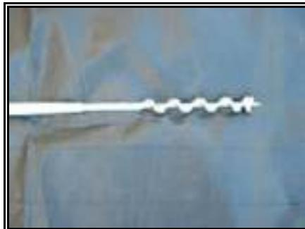
**Figure 13: A typical hand-auger bit**
