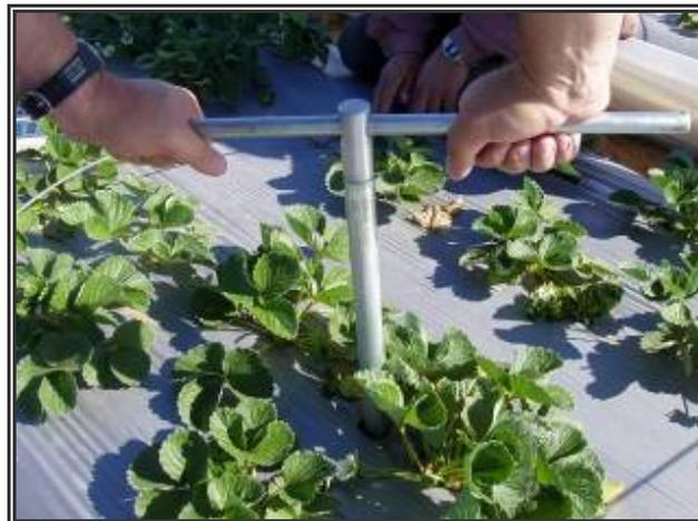
Figure 6: Drilling a hole with the hand-held auger
