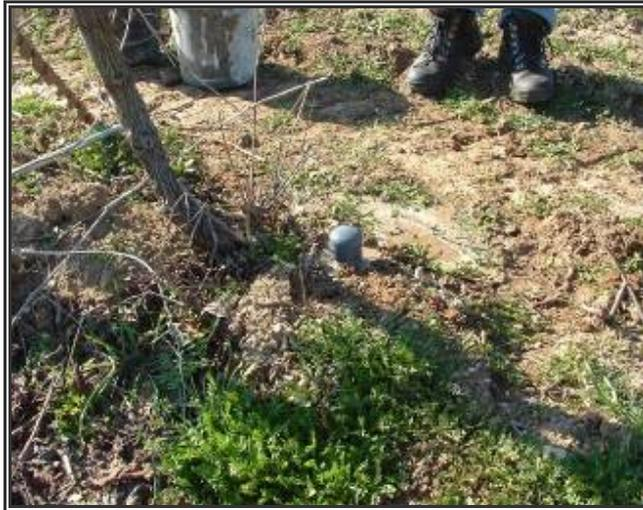
**Figure 12: An installed MobiCheck access tube**
