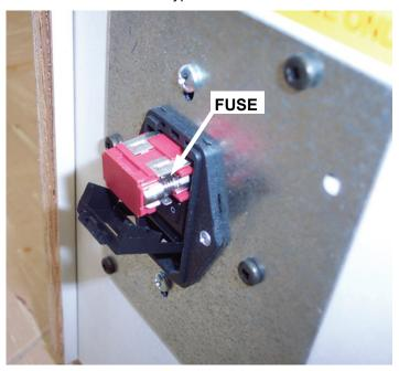
Three fuses are located on the Power Supply PC Board, and one fuse is located on the AC Power PC Board. Using a small flat blade screwdriver, pry the fuse from the fuse holder. Remove the fuse from the fuse holder and test each fuse as required. the fuses. Be sure to replace the fuses with the same type and value.
