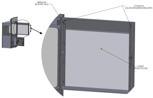
Remove the 8 8-32 Kep nuts that hold the glass retaining bracket to the door. The glass can be removed. Reassembly in reverse order.
