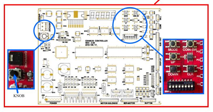
The Mode button found on the main board will allow you to setup your cost of play and also allow you to adjust how far the spider will descend into the prize chute when a prize is won. See the section on Mode options.
