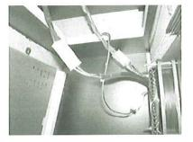
Step 6: Make the following connections: fluorescent lamp power, marquee speaker/LED signal, fan power.
