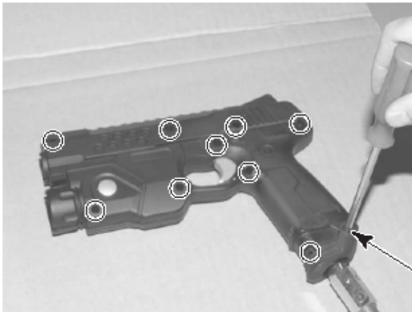
SCREW (10), black M3 x10, w/small flat & spring washers
