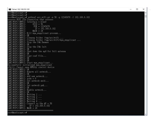
Fig. Set up Wi-Fi connection between DUT and AP
