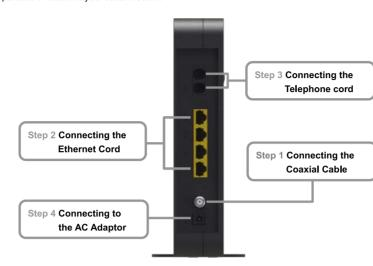
Step 1: Connect a cable by feeding the F-connector on the back of the cable modem. Ensure the center conductor of the 75 ohm coaxial cable is inserted directly into the center of the F-connector. Secure the coaxial cable by carefully threading the outer shell of the coaxial cable connector onto the F-connector in a clockwise direction until tight. Be careful not to over-tighten the connector or you may damage either the connector or the cable modem.
