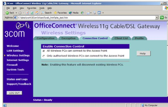
A higher level of security can be achieved for your wireless network if you use both encryption and you specify only certain wireless computers can connect to the Router. By default, any wireless computer that has the same Service Area Name/SSID, channel and encryption settings as the Router can connect to it.
