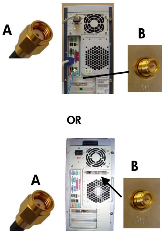
**Figure 1: Antenna Attachment**
