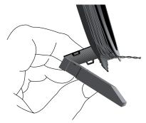
2. Push the tab into the open slot in the base of the stand. Press until the tab clicks home.
