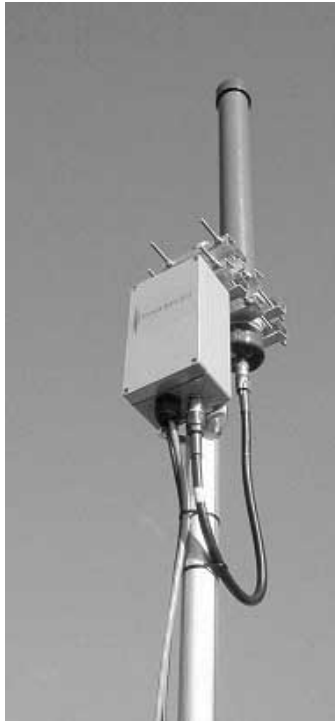
Figure 3-1: Omnidirectional transmitter and antenna.
