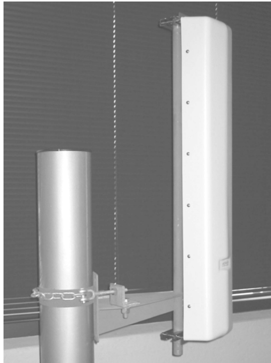
Figure 2-4: Pole-mounted Access Point.
