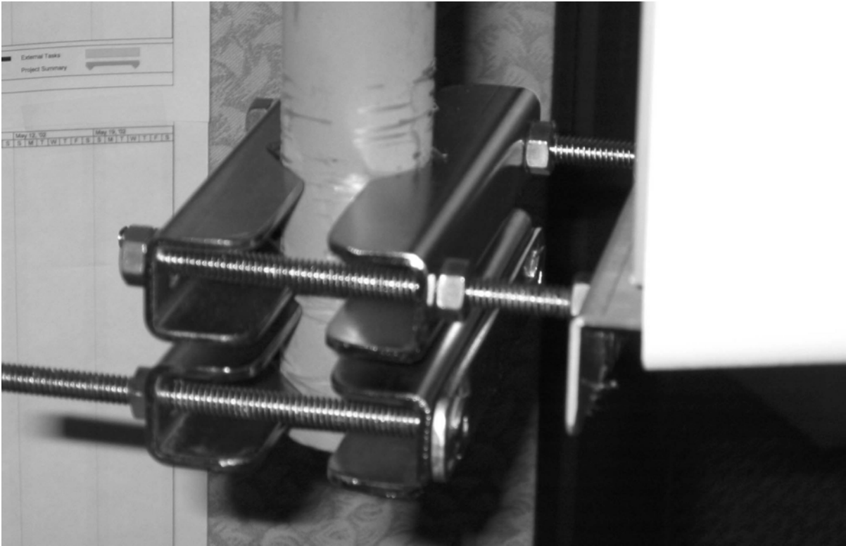
Figure 3-10: Pole Mount with temporary pivot bracket detail.
