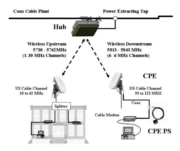
The hub connects directly to the coaxial portion of cable plant using a standard power extracting tap and is line powered over coax using 60 or 90 VAC. The CPE is installed at the customer site, connects to a standard cable modem, and is powered over the coax cable using a wall mounted AC adaptor and DC to coax power inserter.
