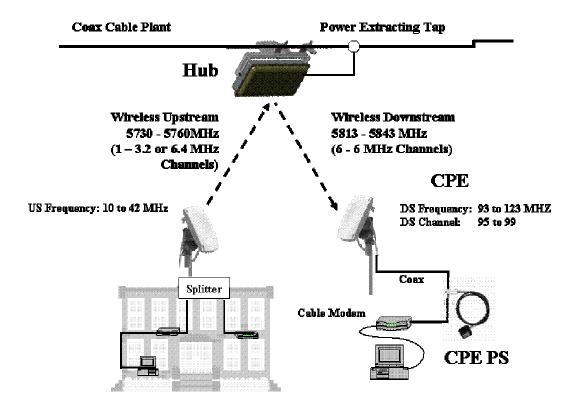
The hub connects directly to the coaxial portion of cable plant using a standard power extracting tap and is line powered over coax using 60 or 90 VAC. The CPE is installed at the customer site, connects to a standard cable modem, and is powered over the coax cable using a wall mounted AC adaptor and DC to coax power inserter.
