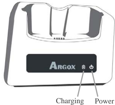
Figure 2-5 The Front of the CRD-90
