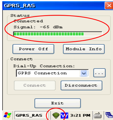
FIGURE 3-44 GPRS SIGNAL STRENGTH
