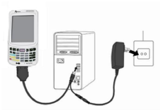
Figure 2-11 Communication through Cable
