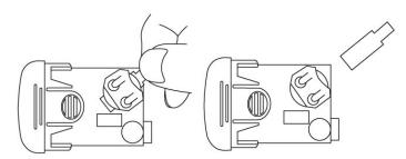
3. Make sure battery is in the slot and close cover back.
