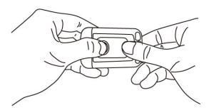
2. Remove battery insulation to start Tag-60 up.
