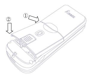
4. Make sure cover is closed and slide two latches back.
