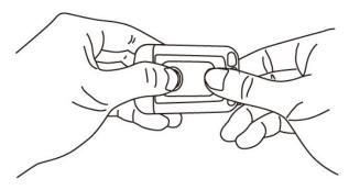
2. Replace CR-2032 coin battery. Make sure positive electrode is up.
