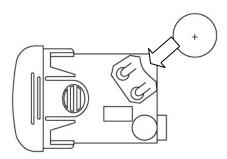
3. Make sure battery is in the slot and close cover back.
