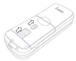
2. Inserting two batteries as indicated inside battery compartment.
