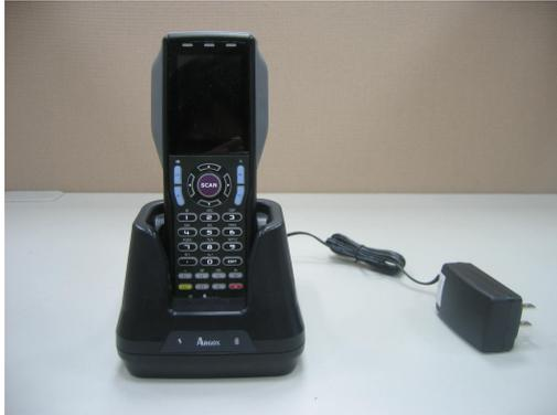
Place the PT-20 into the cradle (first connect the power supply to the cradle)
