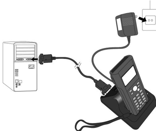
**i** When both RS-232 and USB cables are connected between the CRD-10 cradle and host computer, the USB interface takes priority for data transmission and the RS-232 communication is automatically disabled.
