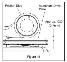
Check the adjustment with the engine off and with the engine on:
