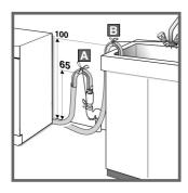
A. Connect the drain hose, without kinking it, to a draining duct or a wall drain fixed at a height between 65 and 100cm from the floor. Use the curved bracket, if reqired.
