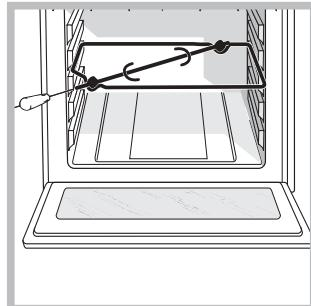
2. Place the rotisserie support in position 3 and insert the spit in the hole provided on the back panel of the oven.
