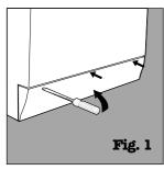
To access this pre-chamber, just remove the panel covering the bottom of the washer-dryer using a screwdriver (figure 1); then lift the cover rotating it anti-clockwise (figure 2) and check its contents accurately.
