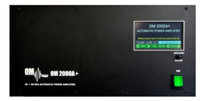
**ON** - **Main Switch.** After turning ON small 12V APU for logic, protection circuits and the display will be activated. High voltage and RF circuits are still OFF.
