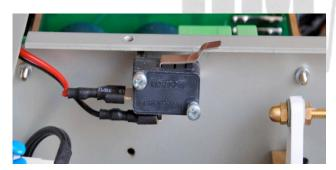
One of the important safety element is mechanical switch for AC blocking at opened amplifier.
