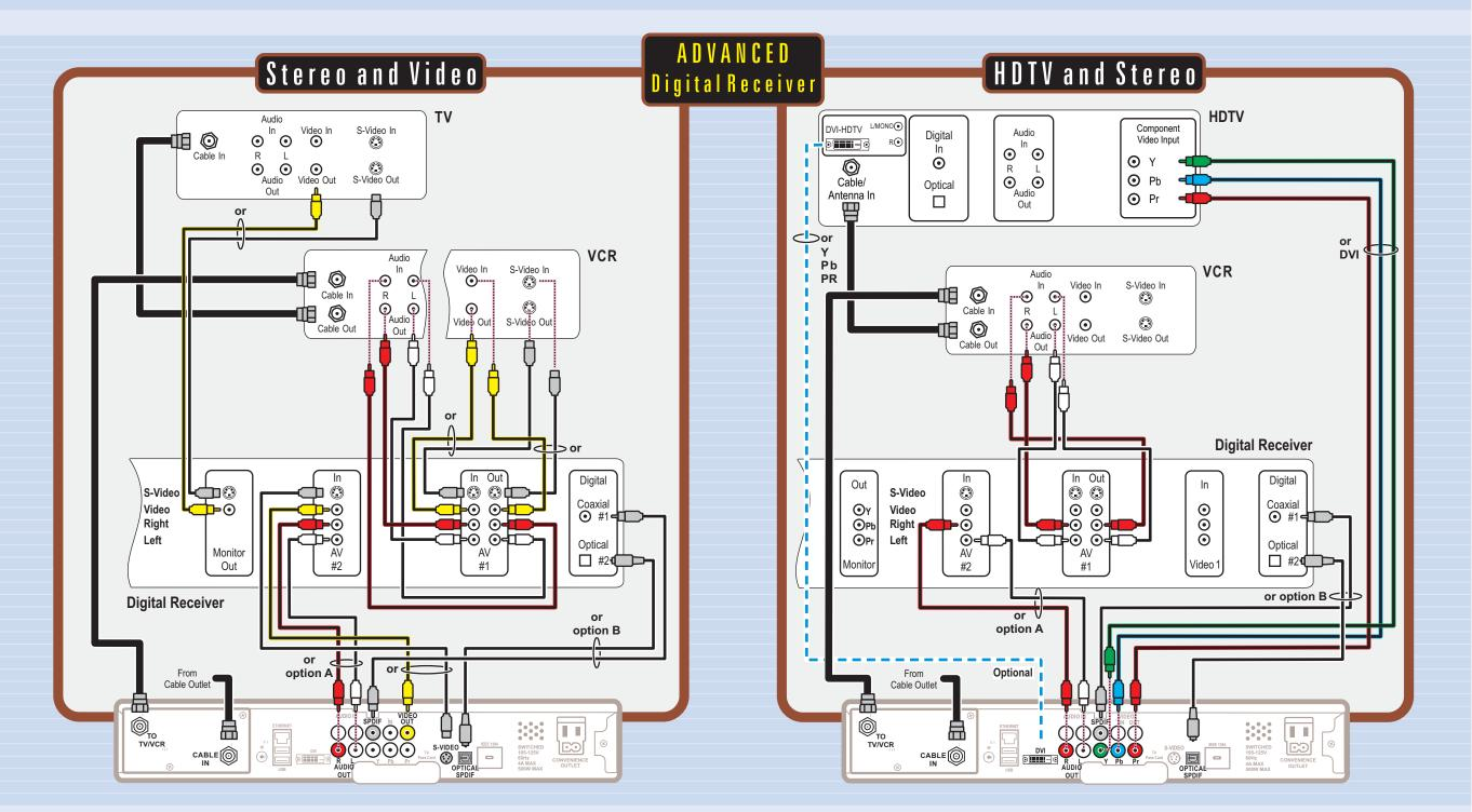
If your DCT5100 and HDTV have optional DVi connections, connect to your HDTV using the DVi cable. Be sure to connect the left and right audio cables to the DVi L/Mono and R jacks on the TV. For more detailed information, refer to the DCT5100 User Guide. Please see the Important Safety Instructions on reverse.
