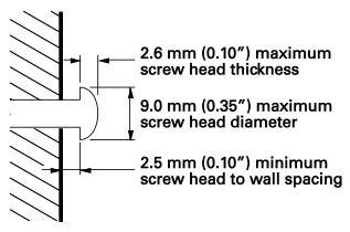
Figure 4: Wall Mount-Screw Head Dimensions
