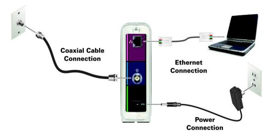
Figure 3: SB6141 Connection Diagram
