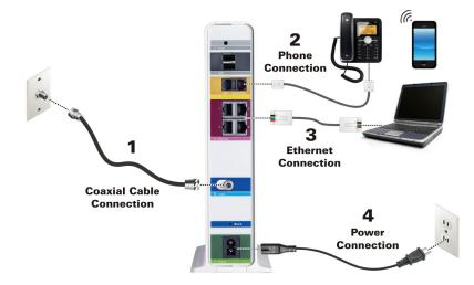
1. Connect the coaxial cable (connected to the cable wall outlet or to an RF splitter) to the **Cable** connector on the rear of your SVG2482AC.
