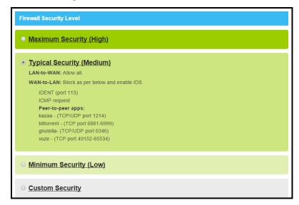
Figure 32: Firewall IPv4 Security Level – Medium Screen
