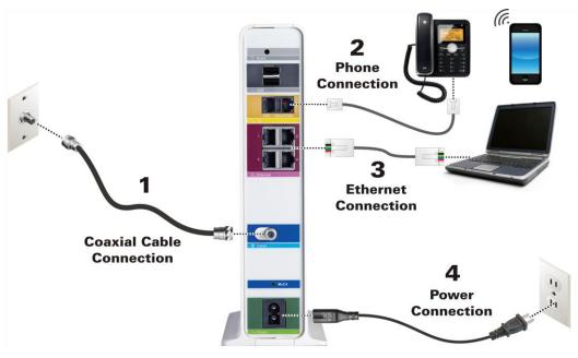
Figure 4: SVG2482AC Connection Diagram
