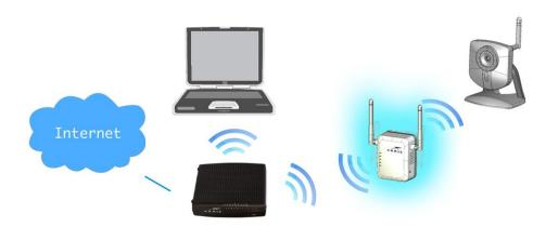
**Step 1:** Locate the WR2100 Wireless Repeater near the Wireless Access Point while doing the configuration.
