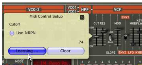
"Cut-off" parameter waiting for the control to be assigned
