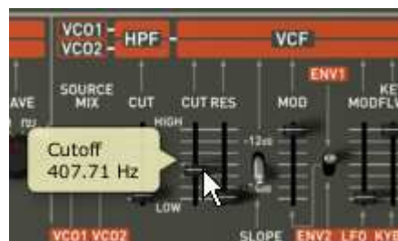
Lower the cut off frequency of the filter
