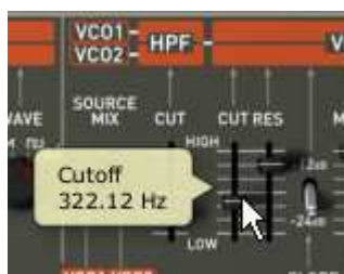
Lower the cut frequency of the VCF
