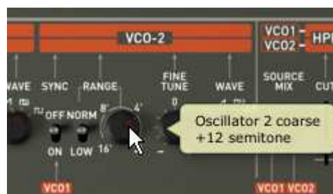
Tuning the second oscillator
