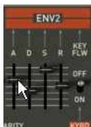
Increase the "Attack" time of the amplitude envelope.
