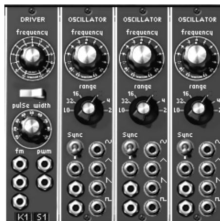
An oscillator bank: 1 "driver" and 3 "slave oscillators"
