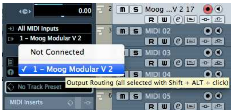
Connection of a MIDI track to the Moog Modular V
