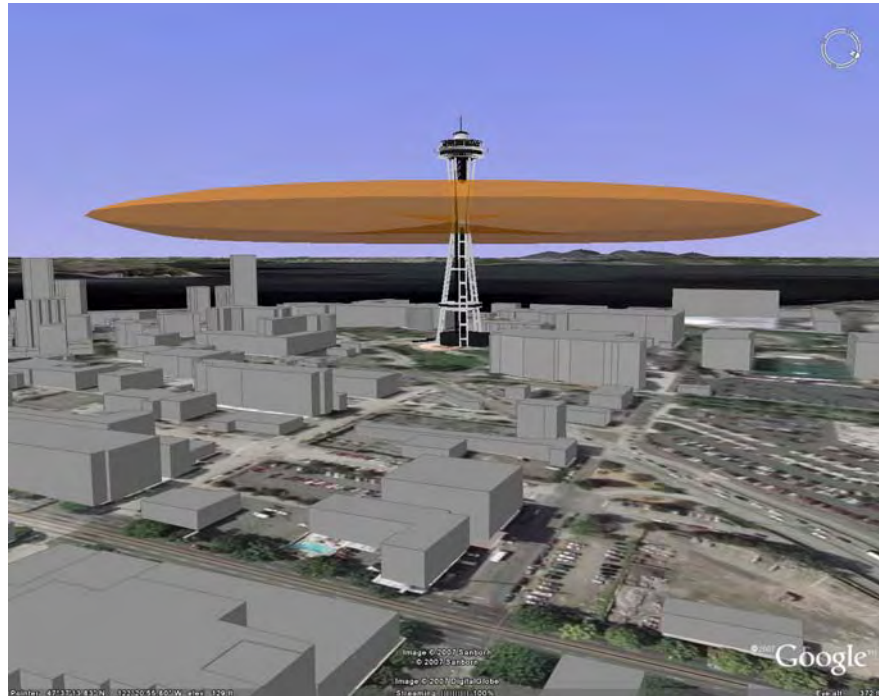
Figure 32 AP-ANT-80 H-Plane View (Top View)
