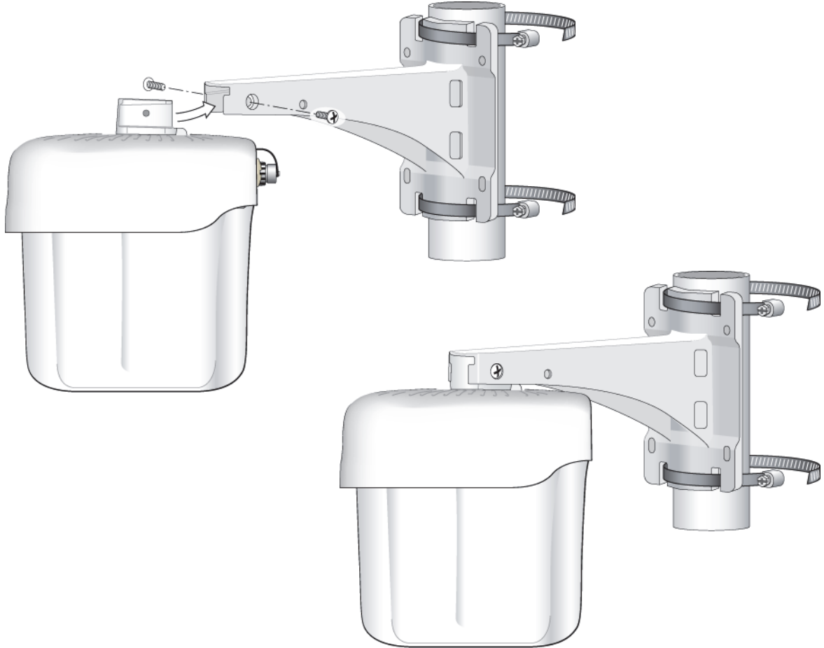
Figure 21 Attaching the AP to the Mounting Bracket (AP-270-MNT-V2)
