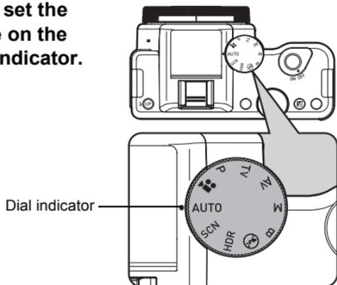
The selected capture mode is displayed on the monitor (guide display).
