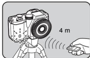
The maximum operating distance of the remote control unit is about 4 m from the front of the camera.
