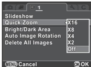
**3** Use the four-way controller (▲▼) to select [Bright/Dark Area] or [Auto Image Rotation], and use the four-way controller (◀▶) to select  (On) or  (Off).
