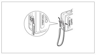
Pass the narrow end of the strap through the strap lug and pass the other end through the loop.
