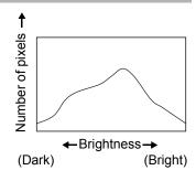
image. In general, when the exposure meter of your image is well-balanced, the graph peaks tend to appear in the middle. On the contrary, when the exposure meter gets imbalanced tending dark and bright without showing a neutral brightness, the peaks appear not in the middle but on both sides.
