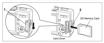
This camera uses an SD Memory Card. Captured images are recorded on the SD Memory Card if a card is inserted ( appears on the LCD monitor) or in the built-in memory if no card is inserted ( appears on the LCD monitor). Make sure that the camera is turned off before inserting or removing the SD Memory Card.
