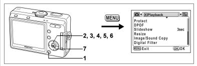
You can copy image and sound files from the built-in memory to the SD Memory Card and vice versa. This function can only be selected when a card has been inserted in the camera.
