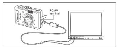
By using the AV cable, you can capture and play back images on a TV or other equipment with a video IN jack. Make sure that both the TV and the camera are turned off before connecting the cable.
