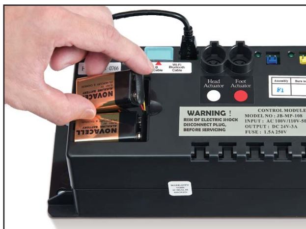
Figure 2: Install 9 volt batteries.
