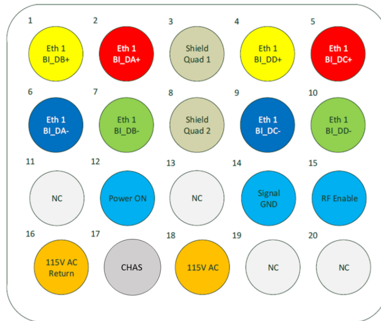
Figure 20: J1 (Pins) Connector Layout and Pin Definitions
