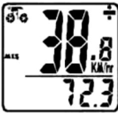
**MAXIMUM SPEED (MXS)**— Maximum speed is indicated by MXS and is displayed on the bottom line. Maximum speed is stored in memory and updates only when a higher speed is reached. To reset MXS, press and hold the SET button for 2 seconds. Now press either MODE button to advance to the Average Speed (AVS) mode.
