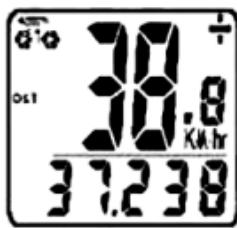
**TRIP METER (DST)**— Trip distance is indicated by DST and is displayed on the bottom line. The Trip Meter is activated automatically with speedometer input (comes on automatically when you begin riding, turns off when you stop). To reset DST to zero, press and hold the SET button for 2 seconds. Note that TM (Trip Time) & AVS (Average Speed) will also be reset at that time. Now press either MODE button to advance to the MXS mode.
