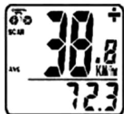
**SCAN**— The Scan mode conveniently rotates DST, MXS, AVS, and TM readings on the computer screen without the need to press any buttons. Now press either MODE button to advance to the Clock mode.
