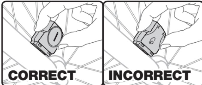
Position the computer sensor on the right front fork so that:
