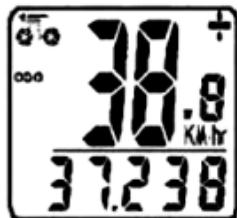
**ODOMETER (ODO)**— Total distance traveled is indicated by “ODO” and displayed on the bottom line. To reset ODO, press the SET button for 2 seconds or remove and replace the battery. Adjust each flashing digit by pressing either the left or right MODE button and then press SET to confirm. Now press either MODE button to advance to the DST mode.
