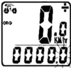
**AUTO STOP/START** – To preserve batteries, the cycle computer will automatically switch off if the unit is left unused for over 5 to 6 minutes. Display will reappear with a press on either button.
