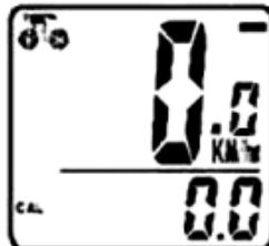
**CALORIES BURNED (CAL)**— This function estimates the number of calories burned while riding, based on the age and weight inputted by the user. To reset CAL, press and hold the SET button for 2 seconds. Now press either MODE button to advance to the (FAT) mode.
