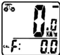
**FAT BURNED (FAT)**— This function estimates the number of fat grams burned while riding, based on the age and weight inputted by the user. To reset FAT, press and hold the SET button for 2 seconds. Now press either MODE button to advance to the (SCAN) mode.
