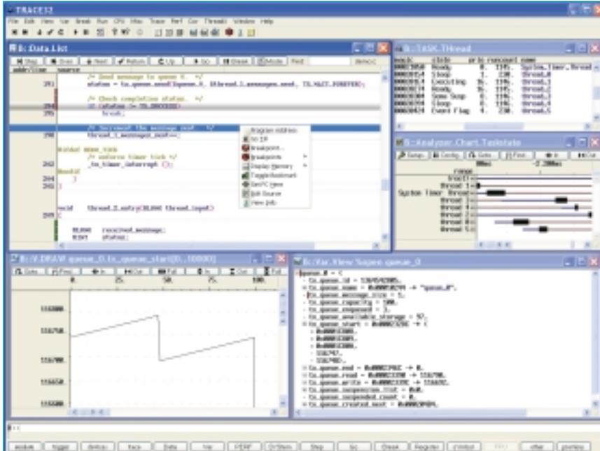
The Graphical User Interface (GUI) **TRACE32-PowerView** is the powerful IDE with the same intuitive look and feel as all TRACE32 Tools. It works together with all third party compilers and can be integrated to editors and CASE-Tools. The complete GUI can be customized comfortably to the requirements of each project. A powerful, easy script language supports you to change the GUI, run test programs or automate command sequences. No other system offers more flexibility.
