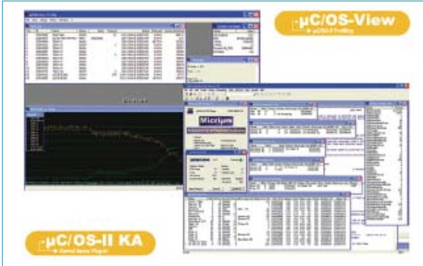
**μC/OS-II** is a portable, ROMable, scalable, preemptive real-time, deterministic, multi-tasking kernel for microprocessors, micro-controllers and DSPs. **μC/OS-II** can manage up to 63 application tasks and provides the following services: Semaphores, Event Flags, Mutual Exclusion Semaphores (to reduce priority inversions), Message Mailboxes, Message Queues, Task Management, Time Management, Fixed Sized Memory Block Management and more.
