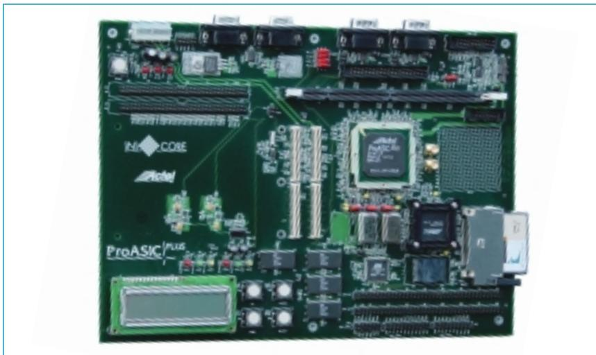
The **SDB-750/1000** is powered by the ARM7TDMI 32-bit RISC processor based AT91R40807. In combination with the 2 Mbytes SRAM and 16 MBytes of program memory (FLASH), the board operates in a standalone mode. It is available with an up to one million gates ProASIC PLUS FPGA from Actel.
