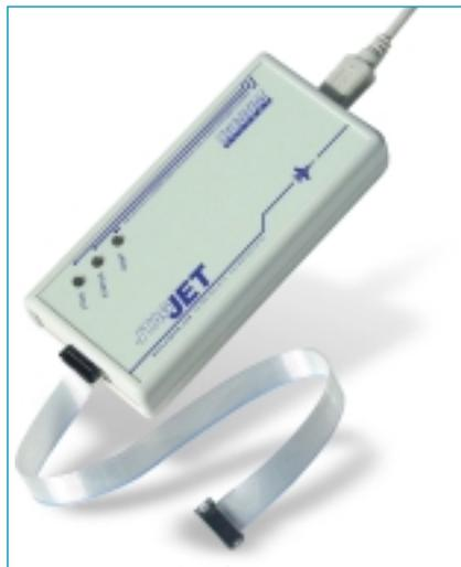
**JTAGjet-ARM** is a non-intrusive In-Circuit Debugger for all AT91 ARM7 and ARM9 based devices. It features:
