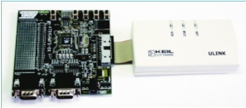
The **Keil ULINK USB-JTAG Interface Adapter** connects the USB port of your PC directly to the JTAG port of Atmel AT91 ARM devices. Using the **µVision Debugger** with ULINK, you can easily create, download, and test embedded applications on actual target hardware.
