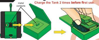
Line up the shapes on the connectors to fit the Tank on the Charging Station. The bright LED will turn on for 60 seconds. Now, the tank is charged. When the LED begins to dim, it's time to replace the batteries.
