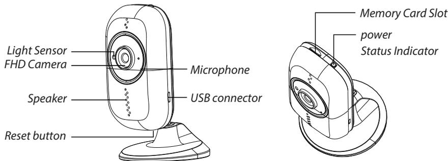
**Note:** Press the Reset for 5 seconds to reset the camera.
