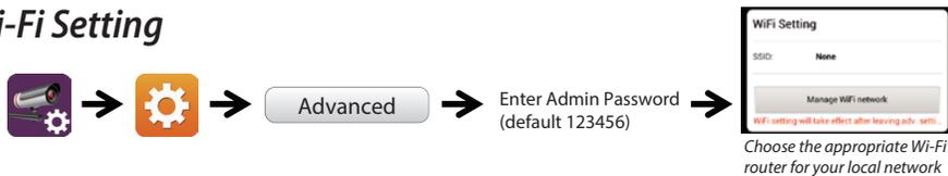
4b. The camera will offline for around 40 seconds to reboot for Wifi connection. When camera connects to wifi router correctly, Green LED will stay ON.
