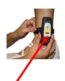
9. Place the WMTD on the offender's leg just below the ankle bone and insert the strap with attached pin tray into the bracket until it snaps in place.
