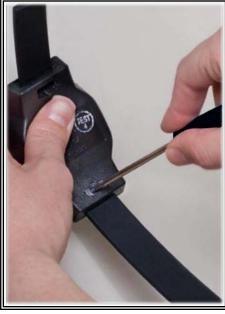
Step 2: Using a Pro Tech flathead screwdriver, push on the tamper plugs to break them.
