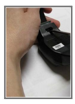
Step 3: Use the screwdriver to remove the tamper plugs from the brackets.
