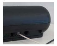
Connect the appropriate end of the power adapter cord into the Power socket located on the rear panel of the SBU2000 Monitoring Unit.
